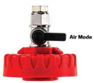
**DRYING - Air Mode:** Turn lever into the horizontal position, pull the trigger and allow air flow to dry the surface, followed by a wipe using a clean microfiber towel. While addressing the surface, work with the Air Pulse Cleaning Gun at 1 inch from the surface and a 45 degree angle.
